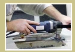
**Step 5 - Profiling:** - Profile the recessed beveled edge using the Alpha® VSP-120 and the Alpha® Profiler EQ-Series. This will create the recessed base for drop-in sinks.
