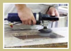
**Step 4 - Grinding:** - Use the Alpha<sup>®</sup> VSP-120 and the Alpha<sup>®</sup> Profiler Z-Series to remove any excess materials remaining. The profiler will create a 90 degree edge.
