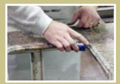
Step 6 - Polishing: - Polish the recessed edge to a high polish with the Alpha<sup>®</sup> Diamond Hand Pads polishing system. These hand pads can be used wet or dry and will create a highly polished rim.
