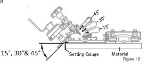
3. Insert the clamps into the grooves on both sides of the guide rail and fully tighten them to the material.
