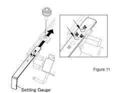
2. Touch both the setting gauges to the edge of the material
