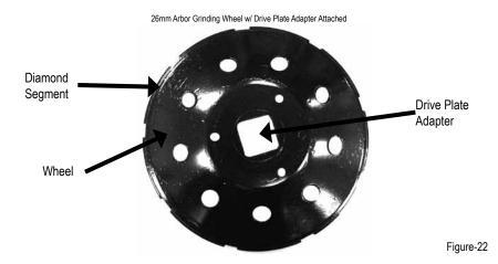
NOTE: The Alpha® 26mm arbor grinding wheel, drive plate adapter and spring loaded flange assembly are designed and engineered to work together. This design eliminates the need for adjusting the grinding wheel height as the diamond segments wear.
