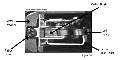
3. Using small needle nose pliers, gently pull the carbon brush holder straight out from the motor housing. After removing the carbon brush holder from the motor housing, you need to remove the power wire terminal from the carbon brush holder (Note: the path of the wire, as it is important for reassembly of the unit). The carbon brush holder assembly is now free from the machine and can be inspected.
