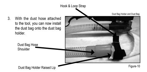
4. Open up the hook and loop strap and slide the hose end into bag until the end of the bag is even with shoulder on the hose end. Tighten the hook and loop strap so the strap is behind the raised lip on the hose fitting.
