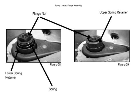
Note: The Spring Loaded Flange Assembly only works with the 26mm arbor grinding wheel (DSQ0500) and the drive plate adapter. A 7/8" round hole arbor will just spin on the flange nut.
