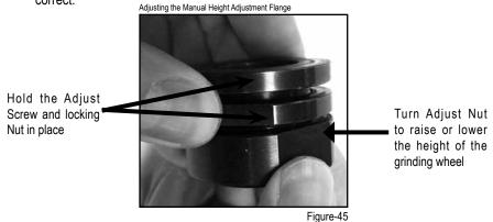
Note: You will need to check the grinding wheel height before each use. As the diamond segments on the grinding wheel wear down, the manual height adjustment flange will need to be adjusted to keep the diamond segments just above (1mm air gap) the top of the brush assembly.
