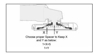
Reference: Example of the combination of Spacer and Base Flange
