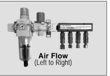
In order to mount the F/R Manifold on the LEFT side of the air drop line, you need to disassemble the unit and re-assemble. Using a 4mm or 5mm hex key, loosen up the hex bolts on the Modular Clamps (#2 and #4) which will allow you to remove all the components of the F/R Manifold. (See Fig. 10)
