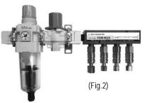
The larger assembly (Fig. 2) has a 1/2" air passageway and is capable of 106 CFM. These F/R assemblies come with four 3/8" NPT couplers, one 3/8" NPT female plug and three 1/4" NPT female plugs.
