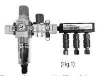
The smaller assembly (Fig. 1) has a 3/8" air passageway and is capable of 53 CFM. These F/R assemblies come with three 1/4" NPT couplers and three 1/4" NPT female plugs.
