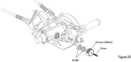
Over time, the Muffler (Part No. 3001-0050) can fill up with oil sludge and will need to be replaced. To accomplish this, the Muffler Assembly needs to be removed, simply remove the Screw (Part No. 3001-0048) and Exhaust Deflector (Part No. 3001-0049) to gain access to the Muffler.
