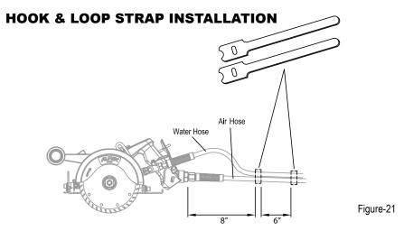
Hook & Loop Straps are supplied to secure both the Water and Air Hose Assembly together which improves maneuverability during the cutting applications.
