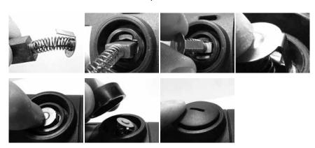
5. Fully tighten the Brush Holder Cap back onto the Brush Holder.
