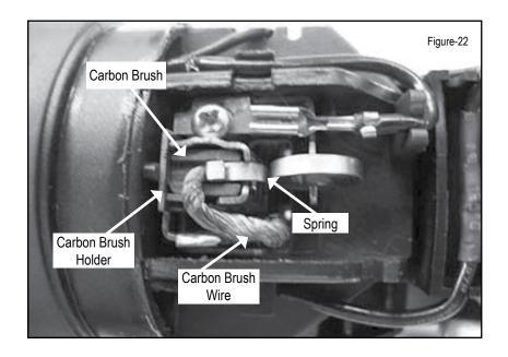
Lift spring from carbon brush and place on the side of the brush holder as shown in Figure 23.
