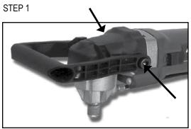
Remove both side screws from center handle as shown in Figure 8.
