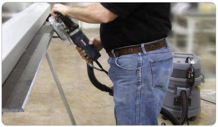
The Alpha<sup>®</sup> Dry Tile Bullnose Kit was designed to create a bullnose edge on tile or stone and polish it to a factory quality finish with a few simple hand-held tools without the mess of dust or water.
