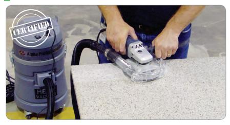
Equipped with a powerful 2-hp motor and an extra large capacity HEPA filter system, the HEPADV10 Dry Vacuum offers the air flow efficiency of vacuums costing three times as much. The certified HEPADV10 is manufactured to the same high quality standards as you expect from Alpha<sup>®</sup>. It includes a high-efficiency 'Drop-in' style HEPA filter individually certified to have a minimum efficiency of 99.97% at .3 microns (based on 1EST-RP-CC007 particle count test method).
