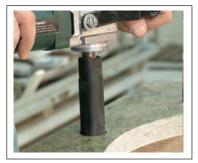
The Alpha<sup>®</sup> Dry Core Bits are designed to drill the faucet-mounting holes in countertops and vanities without using water! Now you can make faucet holes at the jobsite. The bits come in a variety of sizes, and fit on a high-speed angle grinder using the same technique. Alpha<sup>®</sup> makes it easy by eliminating the clean up time needed when using a wet application.
