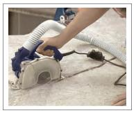
Alpha® Concrete Profiling Wheel - For Creating a Perfect Demi-Bullnose Edge on Concrete Grooves
