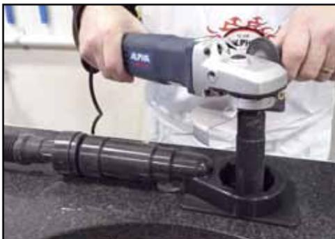
Dust & Water Guard for Core Drilling
