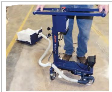
Attach the Alpha® Dust Bag Carriage directly to the Ecogrinder and utilize the Ecogrinder's built-in vacuum system, making the operation simple, easy and virtually dust-free!
