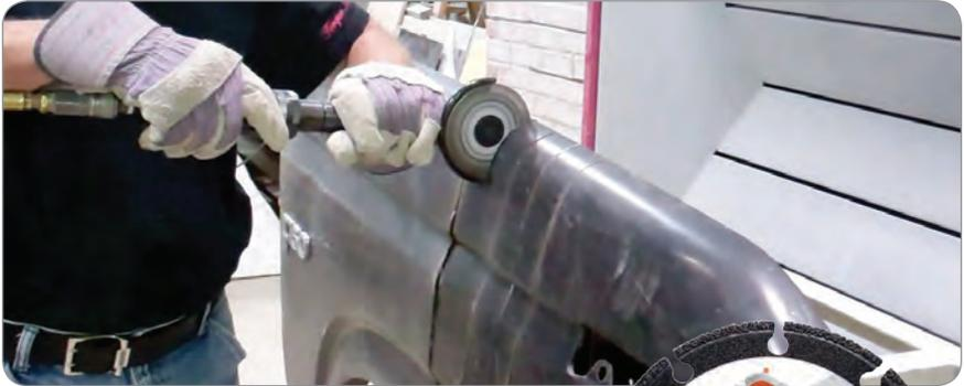
The Alpha® Ultracut ABM Series is designed for use on most popular pneumatic cut-off tools which are widely used in automotive body shops and many other industrial manufacturing facilities. The Alpha® Ultracut doesn't change diameter during the cutting operation and provides maximum cutting depth throughout its life. The Alpha® Ultracut has bi-directional rotation so that you can use on reversible cut-off tools, which could be useful to direct sparks and debris away from the operator.
