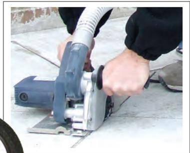
Additionally, Alpha® has combined the Ecocutter, Concrete Profiling Wheel and the Eclipse II Blade to create a virtually dust-free, Concrete Profiling System for creating expansion joints.
