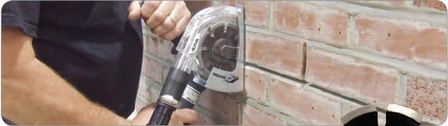
The Alpha® Tuck Point Wheel is specifically designed for brick re-pointing and flash installation. This dry cutting wheel fits on 4", 4-1/2" and 7" grinders. Masons and brick re-pointers will find the Alpha® Tuck Point Wheel to be very aggressive and long lasting. The Alpha® Tuck Point Wheel is segmented with a very hard bond that resists the abrasive mortar commonly used in brick laying. The Alpha® Tuck Point Wheel simplifies brick re-pointing and flash installations.
