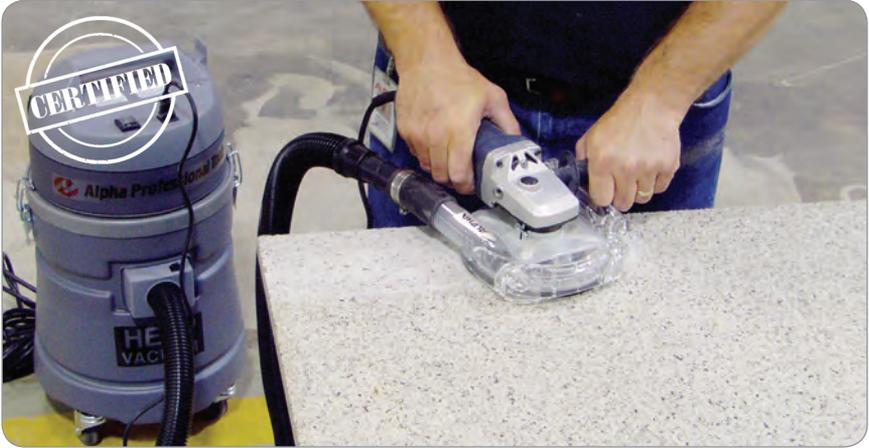
Equipped with a powerful 2-hp motor and an extra large capacity HEPA filter system, the HEPADV10 Dry Vacuum offers the air flow efficiency of vacuums costing three times as much. The certified HEPADV10 is manufactured to the same high quality standards as you expect from Alpha®. It includes a high-efficiency 'Drop-in' style HEPA filter individually certified to have a minimum efficiency of 99.97% at .3 microns (based on 1EST-RP-CC007 particle count test method).
