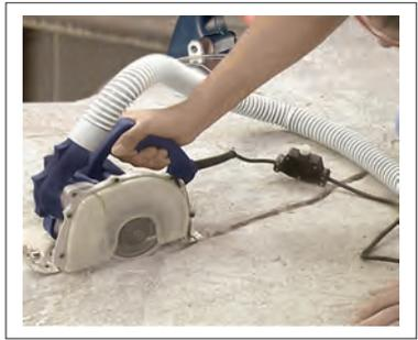
The 4" wheel fits on the Alpha® Ecocutter, thus creating a portable, dust-free operation eliminating unnecessary cleanup.
