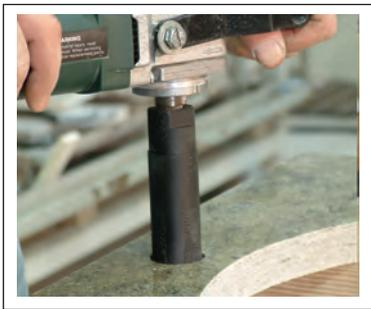
The Alpha® Dry Core Bits are designed to drill the faucet-mounting holes in countertops and vanities without using water! Now you can make faucet holes at the jobsite. The bits come in a variety of sizes, and fit on a high-speed angle grinder using the same technique. Alpha® makes it easy by eliminating the clean up time needed when using a wet application.
