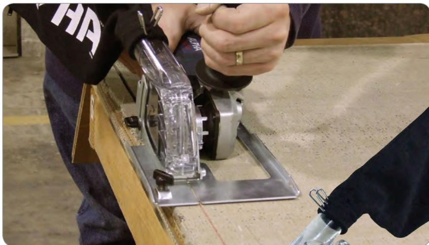
Alpha® introduces the new Ecoguard, designed for collecting dust when using our High-Speed Angle Grinder. The Ecoguard Type C is for used when cutting with dry blades up to 5" in diameter. It is made of high-quality construction for heavy-duty applications. This hybrid dust collection cover eliminates the mess and can be used with or without a vacuum!
