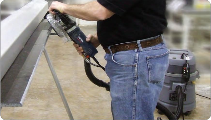
The Alpha® Dry Tile Bullnose Kit was designed to create a bullnose edge on tile or stone and polish it to a factory quality finish with a few simple hand-held tools without the mess of dust or water.
