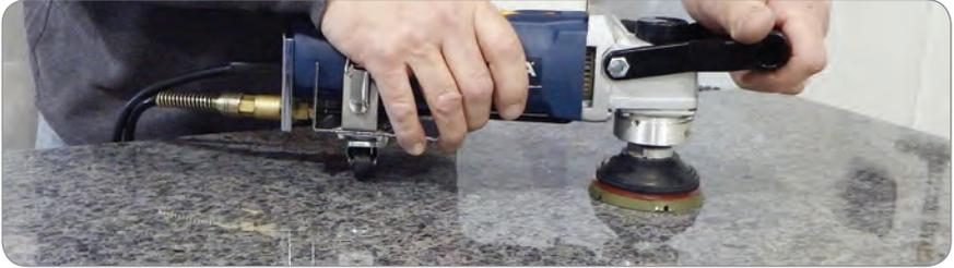
The new generation of electric wet polishers, the AWP-158, is designed for polishing, shaping, core drilling and light grinding. This 7.8 amp, 800-watt, 3,000 RPM machine is a powerful workhorse suitable for use in the shop or on the job site.
