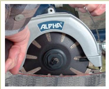
Alpha® Contour Blades are specifically designed for cutting sinkholes and other curve cutting applications on marble, porcelain and harder types of natural stone. The new Alpha® design incorporates diamonds on both sides of the steel core for better performance. The Alpha® Contour Blades fits on the Alpha® AWS-125 wet stone cutter or most common electric angle grinders to provide a convenient, safe and quick operation.
