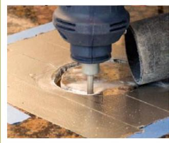
Alpha® Trimmer Bit is very versatile and can be adapted for use in construction trades wherever non-standard shaped cutouts, are needed such as, electrical receptacles, water-valve holes, drains, shower knobs, etc.
