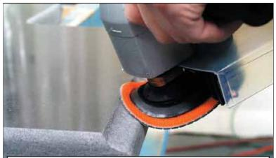
Extra flexibility is required to remove the deep scratches left by the profile wheel on an Ogee edge. Advanced technology makes it possible to follow the delicate curves commonly found on these profiled edges with ease. Ceramica Metal makes even the most difficult edge polishing applications easier.
