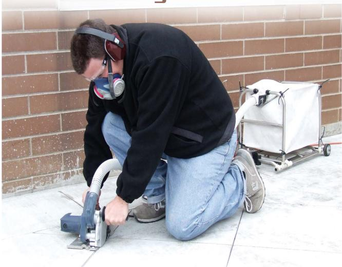
Alpha Professional Tools® has expanded its line of profiling wheels to include the Alpha® Concrete Profiling Wheel. This 3-3/8" wheel is designed to create a demi-bullnose edge treatment on concrete grooves. When used with the Alpha® Ecocutter, it creates the ultimate dust-free portable solution for decorative concrete contractors in the market today!.
