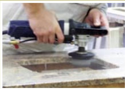
**Step 4 - Grinding:** - Use the Alpha® VSP-120 and the Alpha® Profiler Z-Series to remove any excess materials remaining. The profiler will create a 90 degree edge.
