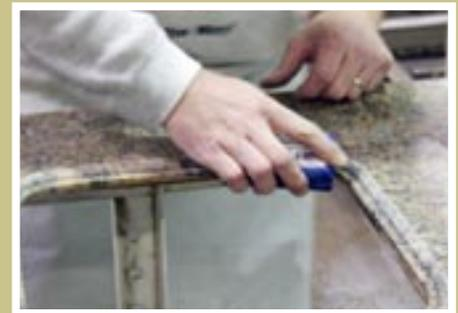
**Step 6 - Polishing:** - Polish the recessed edge to a high polish with the Alpha® Diamond Hand Pads polishing system. These hand pads can be used wet or dry and will create a highly polished rim.
