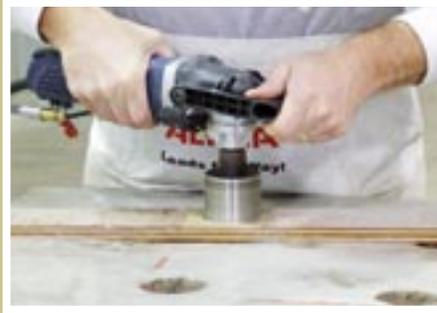
**Step 2 - Drilling:** - Using the Alpha® VSP-120 and the 2-1/2" diameter Alpha® Wet Core Drill Bit, drill holes at the four corners of the cut line in preparation for the sinkhole cut-out. We recommend a template be used when drilling free-hand. Clamp a scrap piece of stone under the stone to prevent excessive chipping on the backside of the stone.
