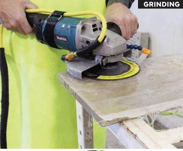
Kit includes: 9" Safety Guard, Loc-Line Assembly, Plastic Tie, 4 Plastic Collars, Adapter (1/4 NPT>>>M10\*P.1.0), Water Hose Assembly, Memory Wrap (3ft. / 1M), Quick Connect Adapter, GFCI Plug (120V), Hook & Loop Tie & Screw w/Spring Lock Washer and Floor Cutting Kit (Part# 510000)
