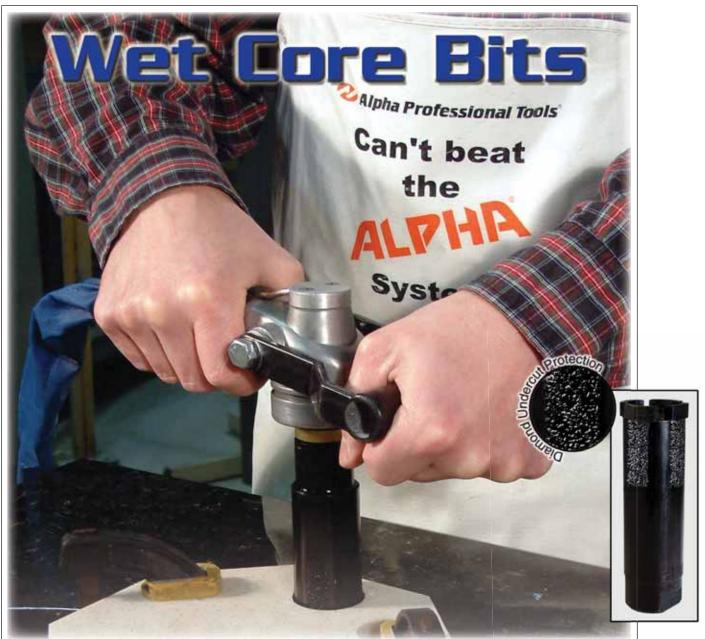
The Alpha<sup>®</sup> Wet Core Drill Bit is designed for drilling the faucet-mounting holes in counter tops and vanities. It can also be used to make clean rounded corners for square or rectangular sinkholes. The Alpha<sup>®</sup> Wet Core Drill Bit is very versatile and can be adapted for use in construction trades wherever holes are needed
