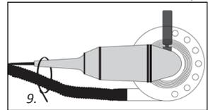
6. The Ecoguard Type EG dust collection cover can accommodate a 1" vacuum hose by inserting the male fitting of the hose into the exhaust port (7) or a 1 1/2" hose by removing the end fitting of the hose and sliding the hose over the exhaust port (7) of the dust cover.
