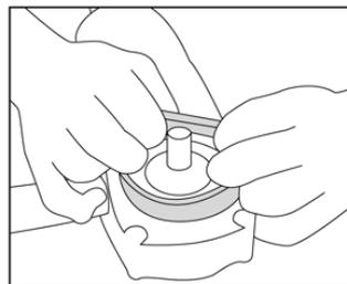
ADAPTER RING - For use on BEARING HOUSINGS (2) less than 2.5"
