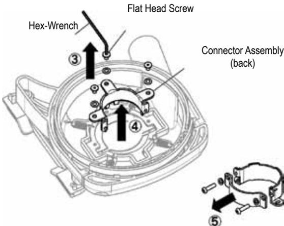
7. Tighten Flat Head Screws with Hex Wrench.
