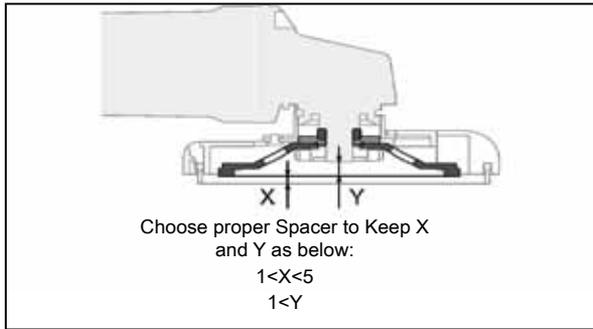
Reference: Example of the combination of Spacer and Base Flange
