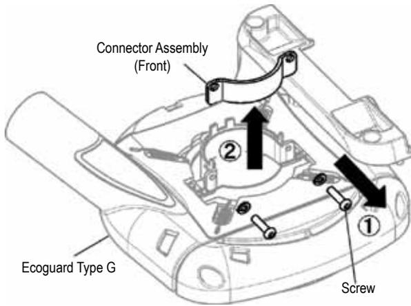
3. Loosen the Flat Head Screws using the Hex Wrench.
