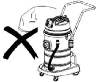
3. Do not force items into the Air Hose Inlet mouth, as it may cause the temperature to rise and damage the motor.
