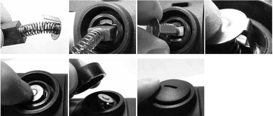
5. Fully tighten the Brush Holder Cap back onto the Brush Holder.
