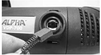
3. Check the carbon brush for wear. Replace if worn down to a 1/4" or if spring is damaged.
