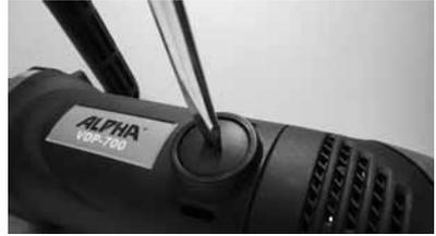
2. Unscrew the Brush Holder Caps completely until carbon brush releases from the brush holder.
