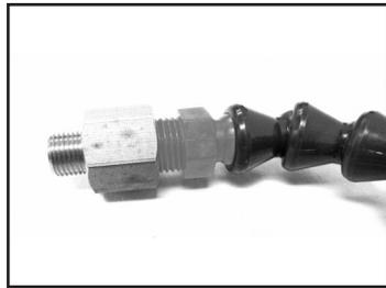
3. Attach and tighten the Water Hose Assembly onto the Adapter.
