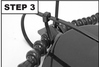
3. Repeat Steps 1 and 2 to completely secure the Loc-Line Assembly to the Safety Guard.
