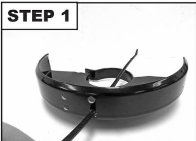
1. Thread Plastic Tie through the drilled holes in the Safety Guard. (If using another grinders safety guard, the guard must be altered to accommodate the Plastic Ties as shown above).
