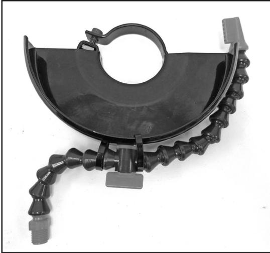
2. Attach and tighten the Adapter on the end of the Loc-Line.
