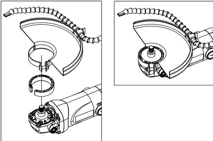
3. Secure the Safety Guard to the grinder by tightening the screw using a screw driver.
