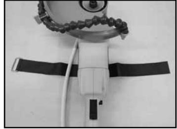
2. Position the Hook & Loop Strap around the Water Hose Assembly and the grinder body.
