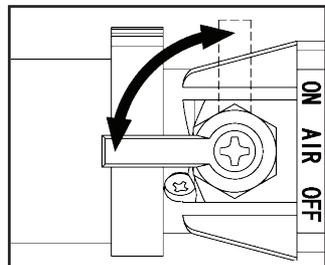
throttle only. Do not attempt to exceed the recommended speed by excess pressure. This will significantly shorten the life of the tool. When storing the tool overnight, disconnect from the air supply and open the valve.
