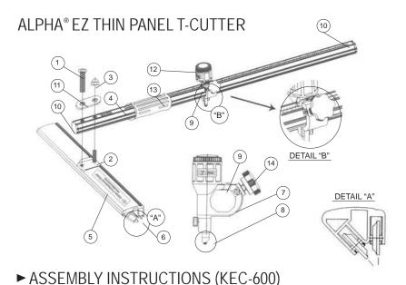
1. Set the scaled bar (4) onto the pre-mounted bolt (2) of the roller housing (5). Make sure that the rollers in the roller housing are in the correct position as the picture. (Detail "A")
