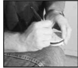
**Note:** Be sure the scale is set to grams, ounce scales will not work for this test. Weigh to the nearest 0.1 gram and note this initial weight on the top of the container label using felt tip pen or permanent marker as well as the time and date the test was started (T1).
