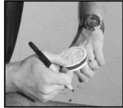
Note the weight as final weight (W2). Do not spill any of the calcium chloride crystals from the container. If any crystals are spilled, the test must be rerun with a new test kit.
