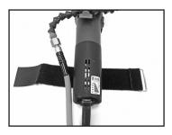
2. Position the Hook & Loop Strap around the Water Hose Assembly and the grinder body.
