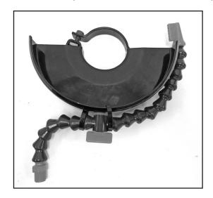
1. Bend the Loc-Line Assembly to conform to the Water Hose Assembly.
