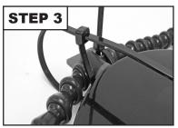
Repeat Steps 1 and 2 to completely secure the Loc-Line Assembly to the Safety Guard.
