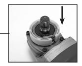
3. Position the Safety Guard over the collar with the shield facing backwards. Push Down until the Safety Guard is firmly seated on the base of grinders neck.
