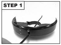
Thread Plastic Tie through the drilled holes in the Safety Guard. (If using another grinders safety guard, the guard must be altered to accommodate the Plastic Ties as shown above).
