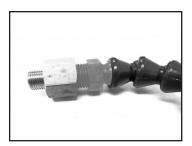
3. Attach and tighten the Water Hose Assembly onto the Adapter.
