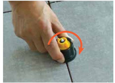
4. Turn Black Base to Tighten
