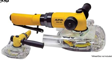
This system is designed for virtually dust-free sanding, grinding, paint and coating removal with up to 5" discs. A removable flat cover allows grinding right to the edge while the dust cover prevents dust from escaping. Also, great for surface preparation, whether it is on concrete, metal, wood, composite or other surfaces. To keep the keep dust to a minimum, an optional water feed system is available.
